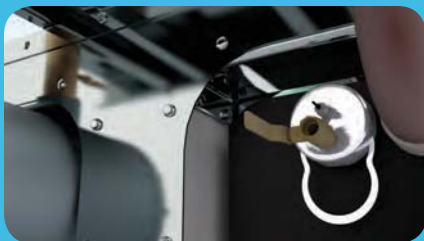
Step 1: Remove containment clip.
