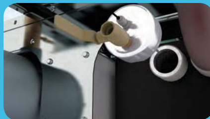
Step 2: Remove strainer assembly cover.
